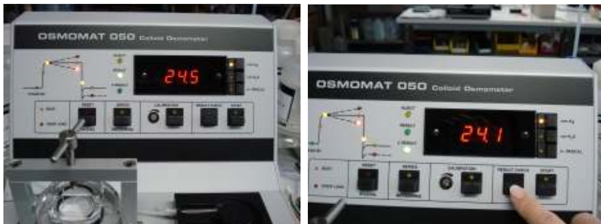
Figure 6-8: Display with adjustment characteristic according to curve 2
