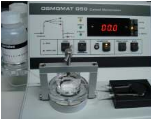
Figure 5-6: Checking the zero point
