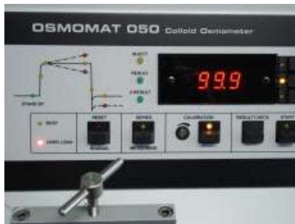
Figure 4-13: Overpressure indicated by "overload" LED
