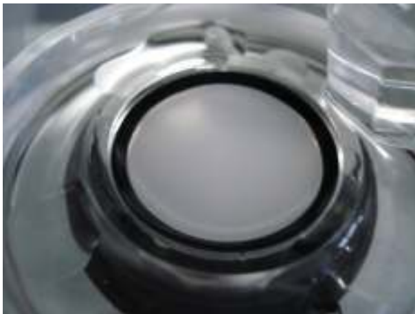
Figure 4-10: Installed membrane and O ring
