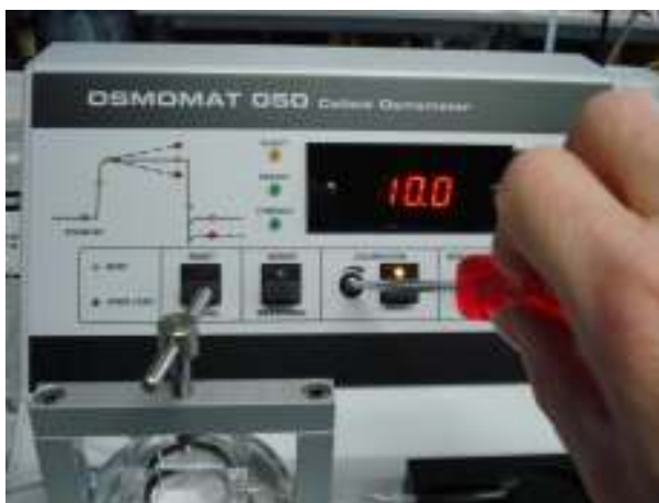
Figure 5-5: Adjustment to 10 cm water column
