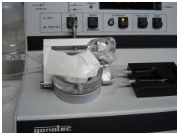
Figure 4-7: Cleaning the lower measuring cell
