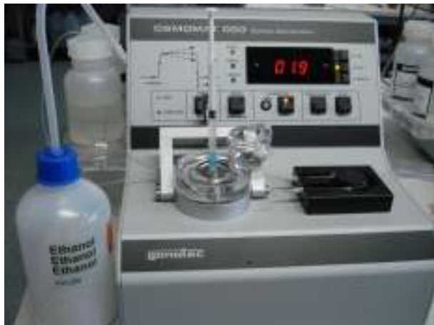
Figure 4-6: Filling the lower measuring cell
