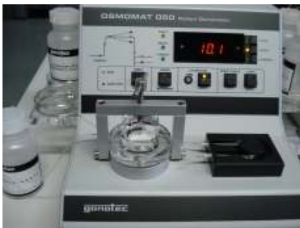
Figure 5-4: Setting the value for 10 cm water column
