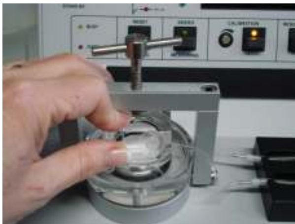
Figure 4-11: Securing the upper measuring cell
