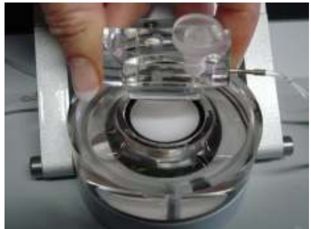
Figure 4-9: Installing the upper measuring cell
