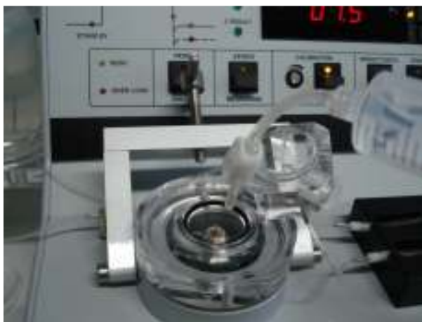
Figure 4-8: Adding the degassed solvent
